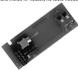
Using external antenna No. 66 99 408, strip the antenna cable, bend the shield backwards onto the isolated part of the wire. The shield should now be mounted in the wire-arrester to secure a good and proper ground plane for the antenna wire. Strip the inner core and place it in the screw terminal.
