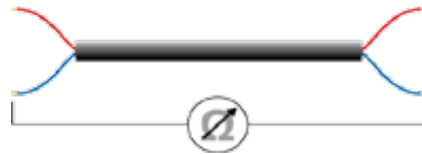
Measurement of cable resistance
