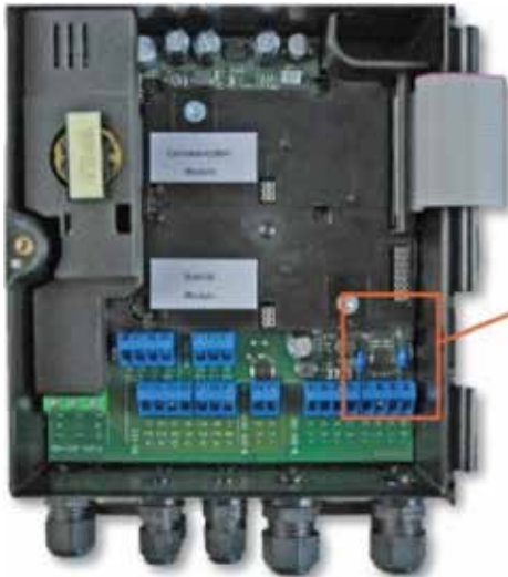
Position of master/repeater jumper
